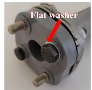
6. Position the shoulder bolts through the large aluminum holes and through the JWest coupler. NOTE: the shoulder bolts will be loose in the aluminum, this is by design to allow isolation and flex. Without this clearance, the parts would be solid metal-on-metal.
